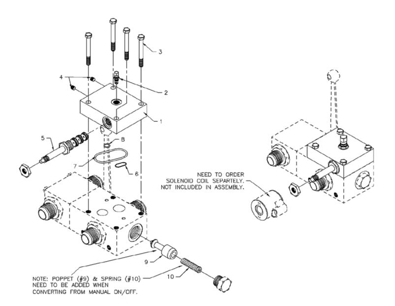
Information For Ordering Solenoid Coil & Connectors: 24 Volt Coil (HF 24 VCD 6353024) – Part #85602000 Din Connect (RR Din Plug RR00011039) – Part #85102790
