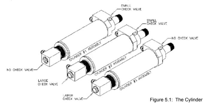
The above figure shows the difference between the cylinder compilation.
