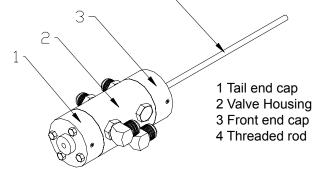
Figure 5.3: The switching valve
