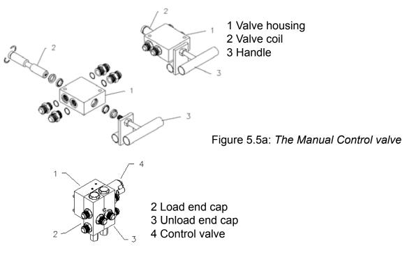
Figure 5.5b: The Electric Control valve1 Pilot valve housing
