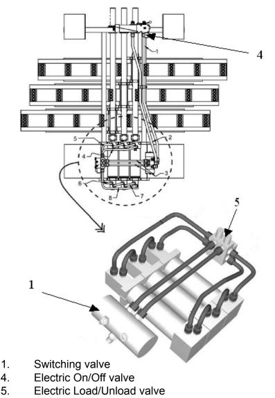
Figure 4.2: Electric operation
