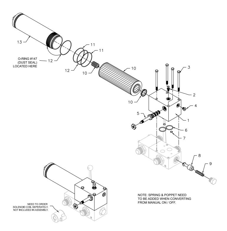
Information For Ordering Solenoid Coil & Connectors: 24 Volt Coil (HF 24 VCD 6353024) - Part #85602000 Din Connect (RR Din Plug RR00011039) - Part #85102790
