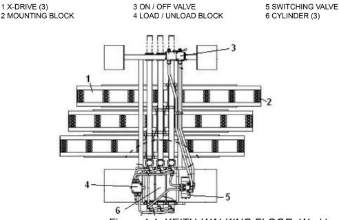
Figure 1.1: KEITH WALKING FLOOR Workhorse drive-unit
