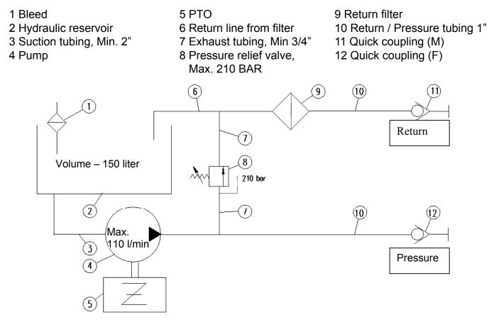
Figure 3.1 Hydraulic diagram
