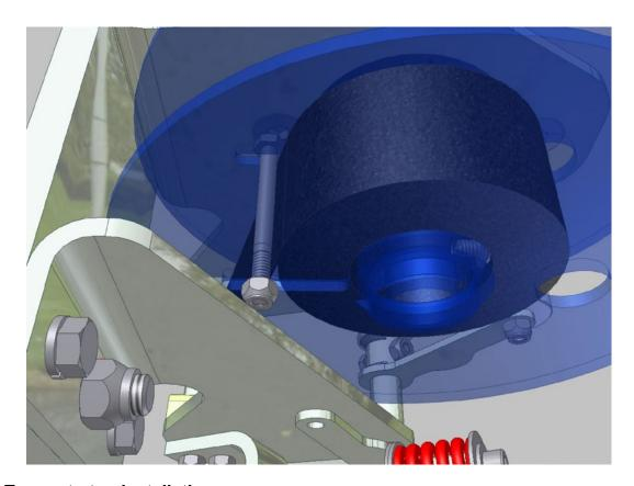
Figure 3: Tarp out-stop installation.
