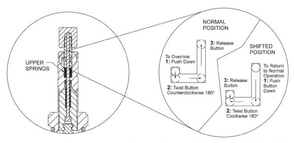
Exaggerated illustration of operation of Manual Override "M" option
