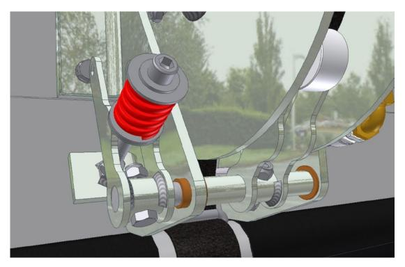
Figure 2: Winch brake
