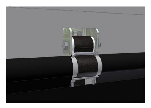
Figure 4: Strap roller assembly mounted at top of front wall.
