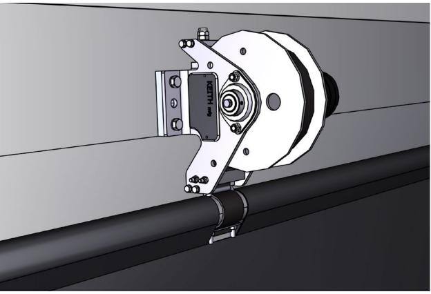
Option 2: Winch mounted at top of trailer front wall (high-mount)
