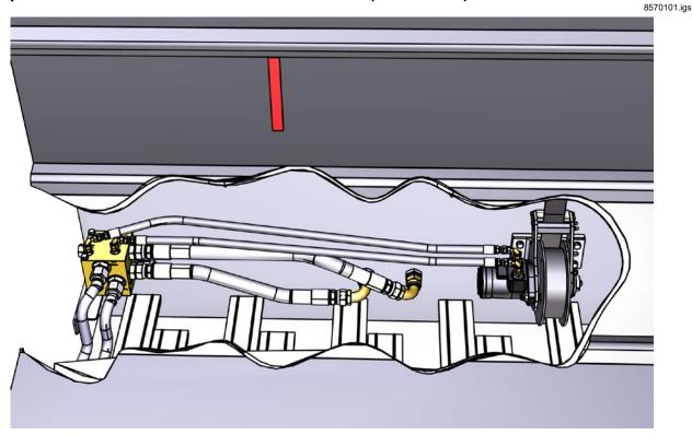
Figure 1: Winch and manifold mounted below the front shield (low-mount).
