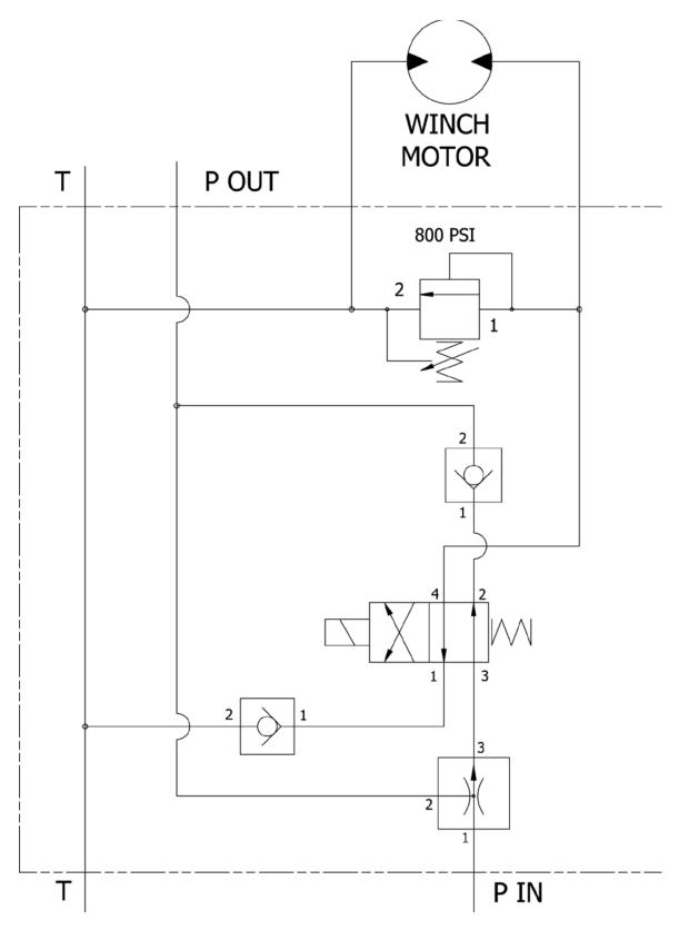
Figure 7: Control manifold hydraulic schematic.
