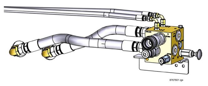
Figure 6: Manifold mounted to exterior front wall on driver's side.
