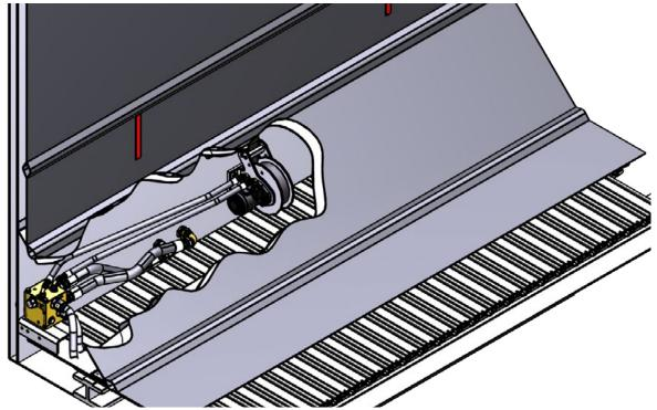
Figure 5: Manifold mounted below front shield.
