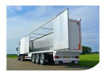
Self-supporting construction with side opening of 6.8m
