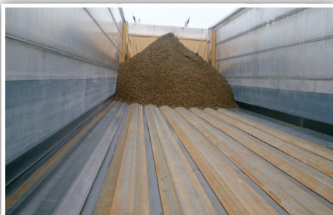
Aggregate material on the plow, first bucket of material needs to be dumped directly on the plow.
