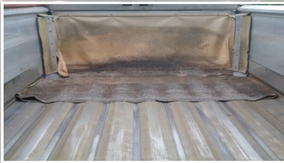
Plow shown in full forward position, sheets laying flat on the floor
