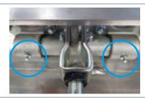
Lubricate with a grease gun.
