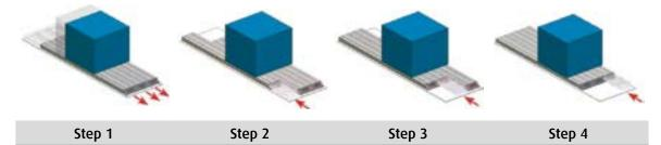
The entire moving floor simultaneously slides in the chosen transport direction by means of the 3 hydraulic cylinders and transports the load
