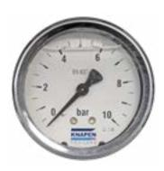
Indication of the pressure in the bags with corresponding weights. This depends on the type of axle and air bags. The settings can be found on the Wabco sticker. For position see chapter 2.2
