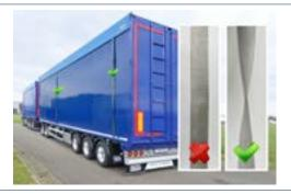
When tensioning the straps, they will rub against the side wall and bottom edge. Protective parts in good condition are therefore required. To prevent paint damage, replace worn protective parts immediately.
