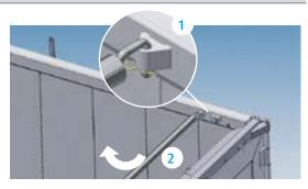
Lift the bar out of the block, turn the bar towards the holder and replace the locking pin. Never turn away all the bars at the same time
