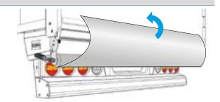
**Rolling up:**Connect the air wrench to the designated air connection. Gradually squeeze the air wrench to roll up the sheet again
