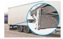
Each light cover contains a sealing rubber to protect against moisture and polution. A proper seal is crucial for the life of your lighting system.
