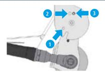
To switch between positions, simply pull out the knob and turn the bracket to the desired position.
