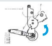
Tighten the wing nut well and use the rotation block to prevent the tube from turning while driving.
