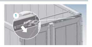
Unlock the locking device on the underside.
