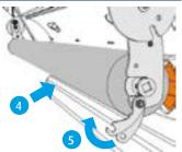
When closing the tube holders, the rotation blockage must remain open so that the roll-up sheet can turn (6).
