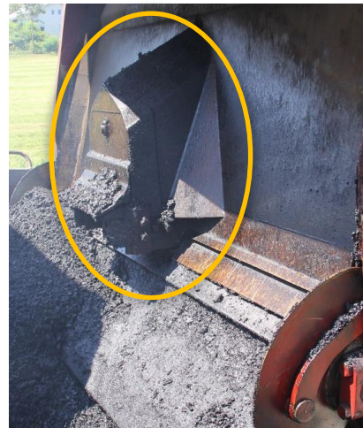
Fig. 58: Closing the rear panel
