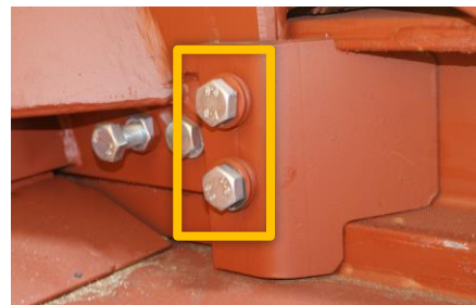
Fig. 98: Adjusting the scrapers
