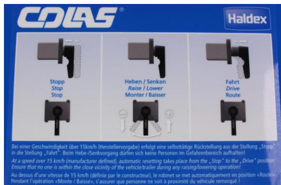
Fig. 29: Raising and lowering with air suspension
